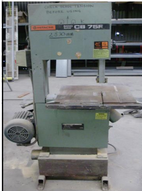
BANDSAW Hitachi. 3-phase. With splitter set-up. 39cm throat. 4-pole motor. 5.5hp. $1990
